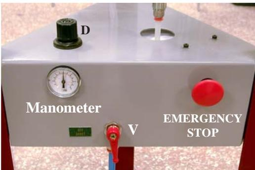
The CS 89 is to be connected to the air source under its lower grey plate, at the level of air valve V. Then turn the air valve V to ON. Make sure that the air pressure shown on the manometer is 6 bar (85 p.s.i.) otherwise correct it with the regulator D.
