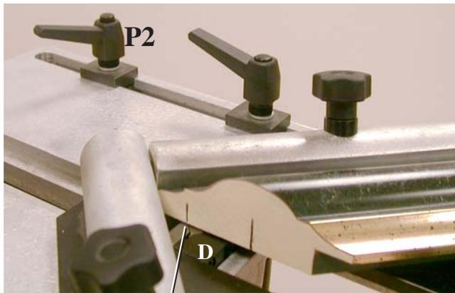
Position the first moulding against stop B1 and slide it up to stop B2.
