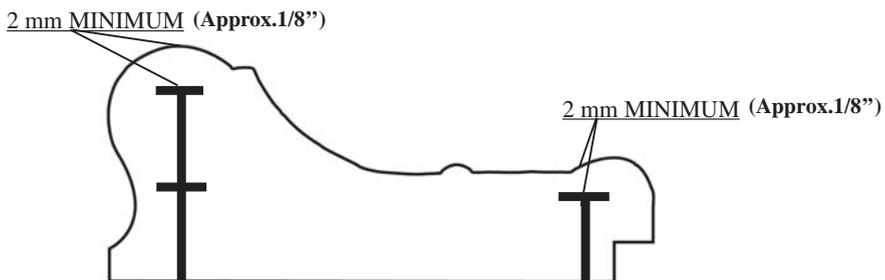
**As a general rule a MINIMUM 2 mm clearance (less than 1/8") above the wedges shall be respected.**
