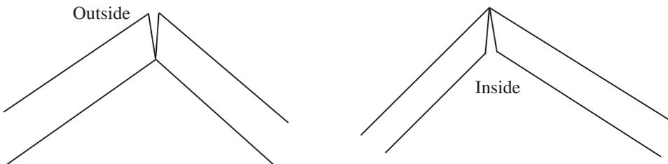
**If the corner is open towards inside, screw in (turn clock-wise) the angle adjustment screw AS (Fig 1 page 1) to correct the fault.**
