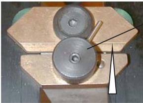
Unscrew the knob of the top clamp, then move the rebate clamp against the 2 mouldings, without forcing. Lock the rebate clamp knob again, without pushing it. Clearance of around 1 mm is left to make it easier to move the mouldings during assembly.
