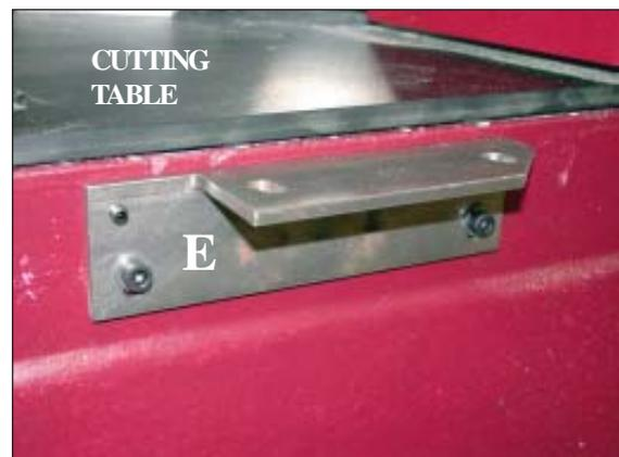
Take the NS out of the crate and turn it over. Place the bed of the NS on bracket E, and screw them together (10mm long tubular socket wrench + 5mm hex head key) **without tightening**, using the 2 screws, 2 washers and 2 nuts provided.
