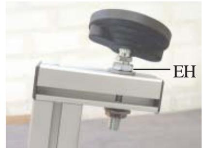
After adjusting level alignment, tighten the nuts of bracket E permanently (10mm tubular socket wrench + 5mm hex head key). Remove the alignment nylon wire. Insert the plug at the end of the aluminium profile.
