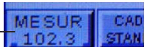
If the button is pressed, the moulding measurement will be displayed in the field: **LRG MOUL (moulding width) (102.3 for example).**
