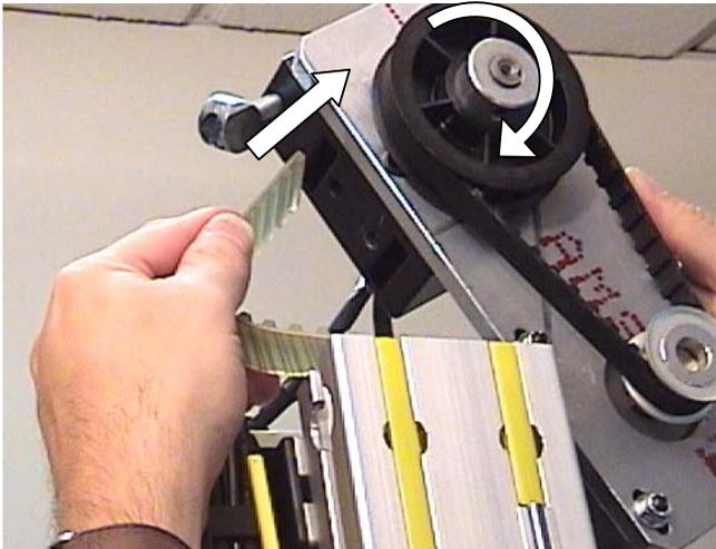
Insert belt into left slot in reversing unit
