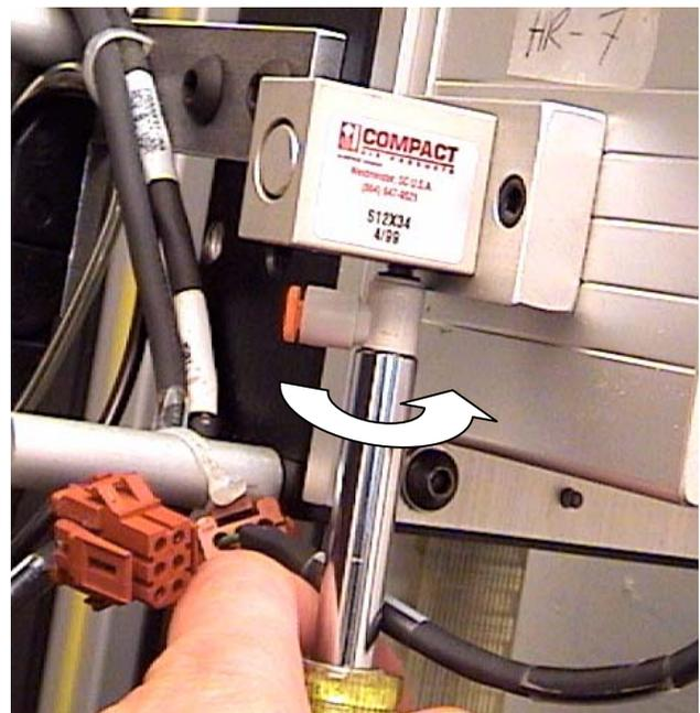
the hose fitting portion of the valve to the left in order to face it toward the air hose. Use caution not to over tighten the valve or hold the tool at an angle that may cause the threaded portion of the valve to accidentally crack or shear off.
