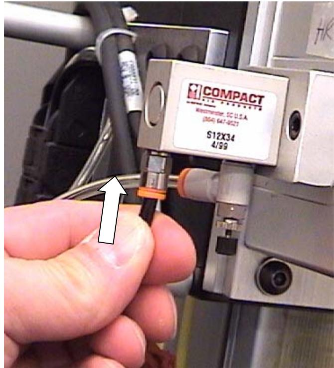
9) Re-connect the main air hose to the machine. Make a test cut and check for acceptable amount of over-cut. Open the adjusting knob (CCW), to lengthen the Start of Cut, and close the valve (CW), to reduce the Start of Cut or slow down the rate of blade plunge. Be sure to tighten the knurled silver lock ring once you have achieved the desired plunge speed / over-cut.
