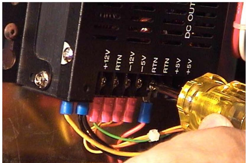
Use a “stubby” Philips screwdriver to loosen terminal screws
