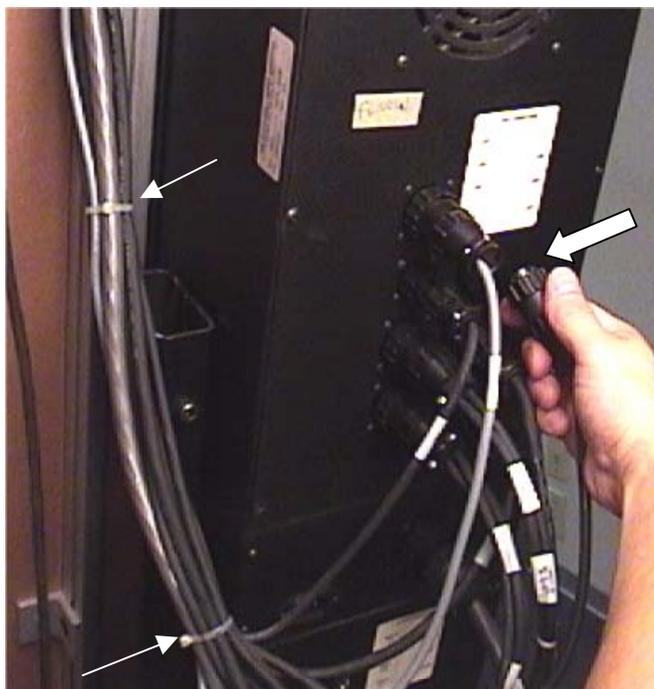
**Unplug C-motor cable and cut cable ties**
