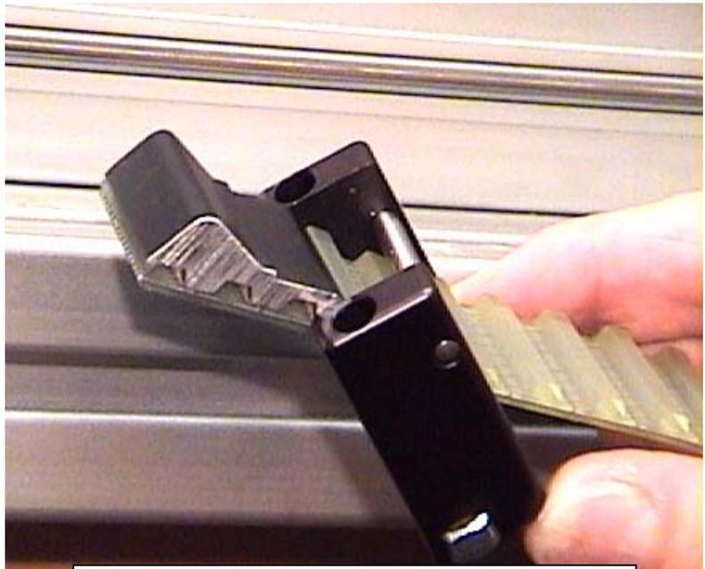
**Proper location of belt wedge in coupling**
