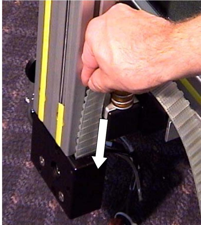
**Note:** You may need to remove the upper reversing unit from the top of the Y-gantry beam in order to thread the belt through it. Loosen and remove both recessed universal fastener bolts from the top end of the gantry with a 5mm Allen wrench. Carefully support the weight of the Y-axis motor and lift the reversing unit off the Y-gantry. You may also feed the belt into the top reversing unit first, and remove the lower unit from the gantry instead.
