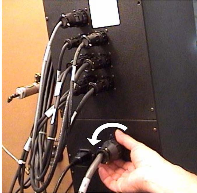
4. Disconnect the connectors (monitor, keyboard, mouse, printer, *if present*) from the lower rear panel of the enclosure. Loosen thumbscrews on the monitor and mouse connectors and pull straight out.
