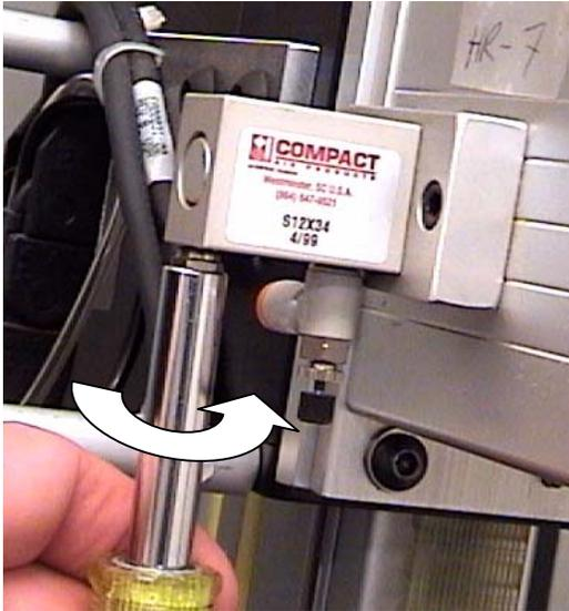
7) Insert the quick disconnect fitting into the cutting head hole nearest you, where the original flow control valve had been mounted. Tighten this fitting with the 5/16" nut driver as well.
