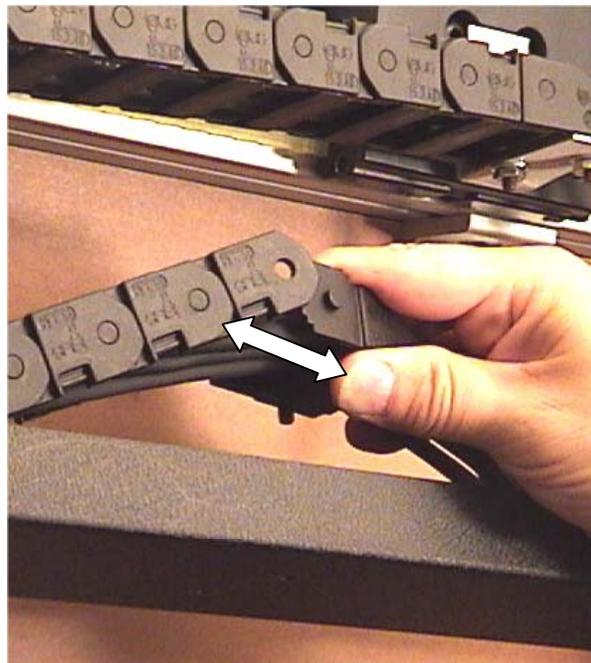
9) Remove the cable connector from the rear of the electronics enclosure, in this case #205 for the C-axis motor cable. Follow the cable back to the X-axis cable carrier, and cut any zip ties holding it in place.
