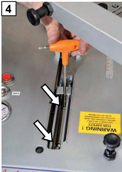
4. Remove the 2 Allen screws.
