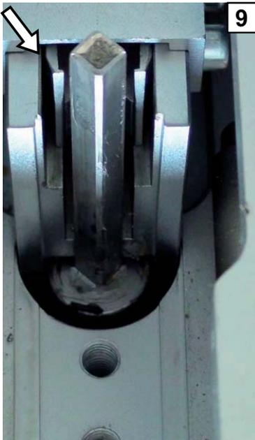
9. NB: align the hammer so that the high part of the piston has the 2 raised sides pointing towards the magazine.
