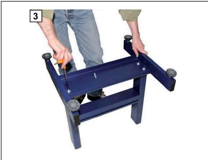
3. Join the base to the uprights using the 4 screws provided
