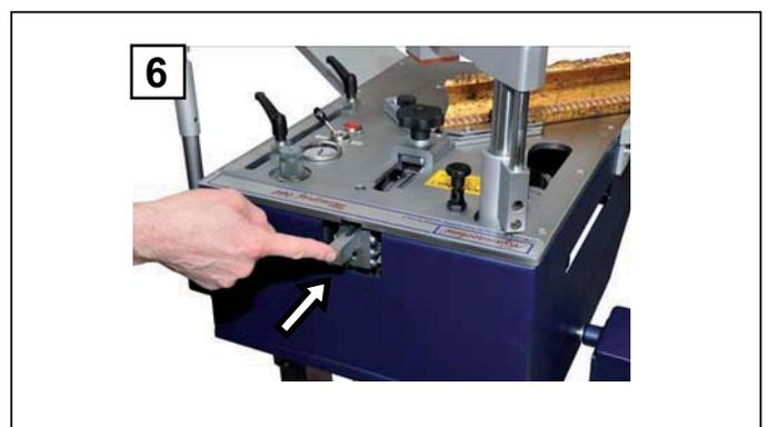
6. Press the cartridge in fully until it locks into position.
