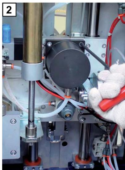
2. Disconnect the 2 pipes connected to the cylinder
