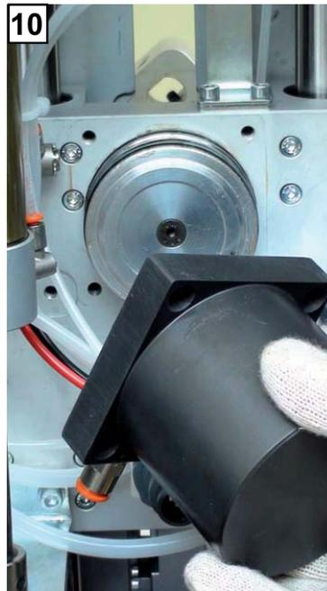
10. Replace the cylinder and push it well up against the head. Tighten the 4 screws and reconnect the air lines.
