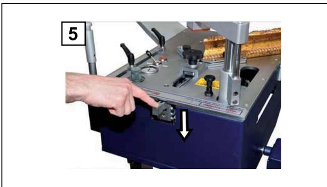
5. Insert the new cartridge in the magazine, keeping it slightly slanted and then press it downwards.
