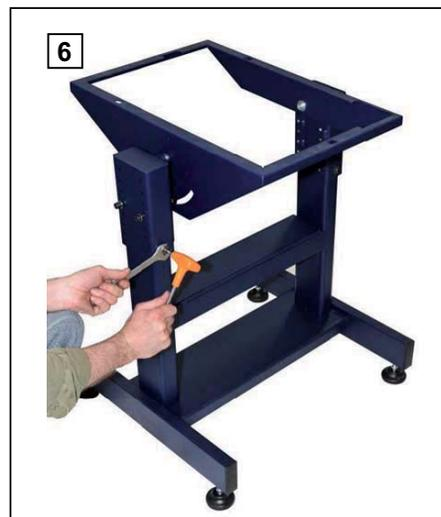
6. Tighten the grub screws and lock nuts.
