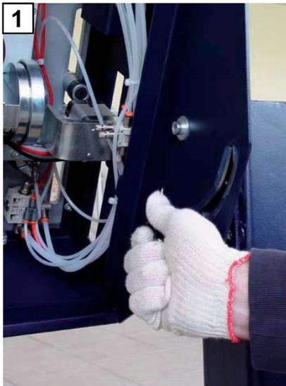
1. Slacken the locking handle on the support stand to tilt the working bench backwards.
