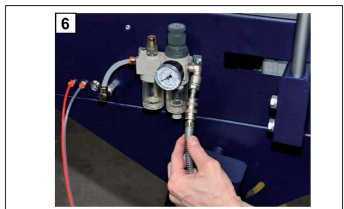
6. Connect up the compressed air supply and adjust the pressure to at least 6 bar, checking the reading on the pressure gauge.
