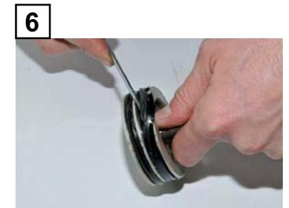
6. Remove the seals from the hammer, clean well and grease, check for signs of wear and/or splintering.
