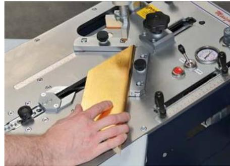
Keeping the positioned mouldings still with your hands, press the pneumatic pedal to activate the front locking clamp. Movement of the front clamp will block the mouldings against the fences so that one hand is now free to take hold of the handle to control the following operations.
