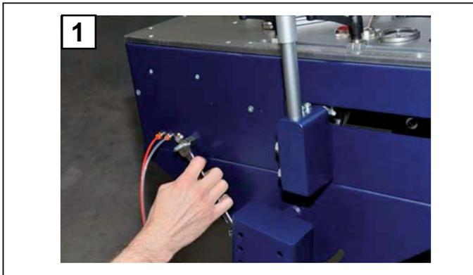
1. Remove the quick-fit connector.
