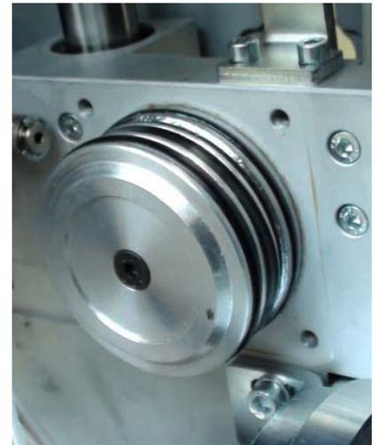
8. Grease the hammer piston and seals well then insert in the relative hole taking care not to pinch the lip seal. If insertion proves difficult, it is advisable to remove the L-shaped support, the head and V-nail cartridge.
