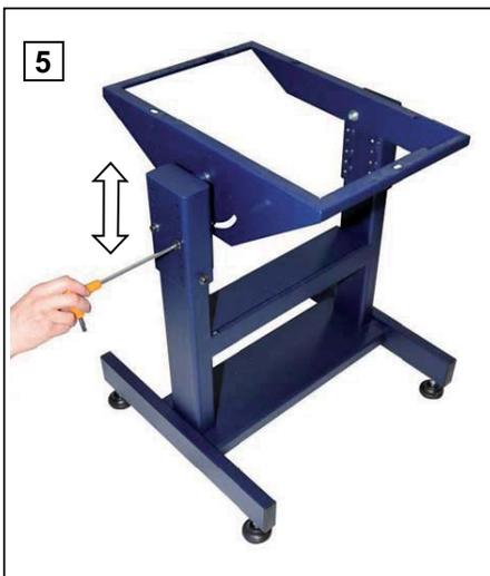
5. Adjust the height as required and then tighten the Allen screws.
