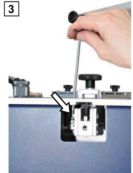
3. Remove the screw which fastens the magazine to the V-nail pusher pneumatic actuator.
