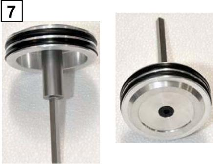
7. If the hammer is worn out or splintered, proceed to replace the whole piston. The raised ends of the hammer must have marked edges to ensure correct insertion of the V-nails.
