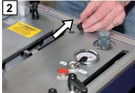
2. Remove the plug from its seat.
