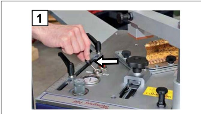
1. Switch the PLV valve (1) lever to the OFF position to open the V-nail pusher.
