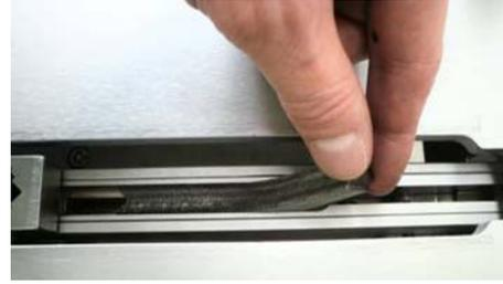
Insert the compressed air line directly into the machine or filter unit (if installed).
