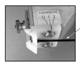
1/16" ALLEN WRENCH The blade support screw keeps the blade stable during the cutting process.
