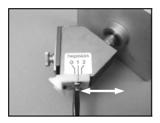
The pressure foot may be adjusted to obtain zero over cut in the corner of the mat. The foot is set on "1" for 4 ply mats and "2" for 8 ply mats.
