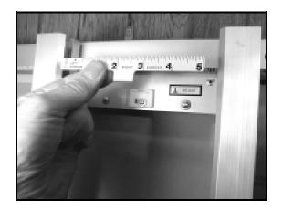
The rule pointers may be changed quickly. Pull the rule pointer straight out from the white plastic bracket.
