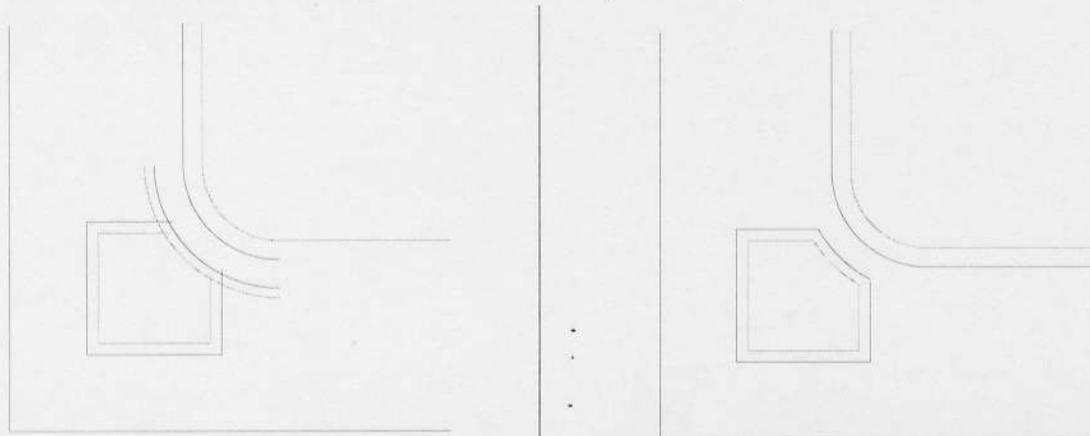
Looks kind of messy at this point, I know, but we can clean it up in a hurry with the "create a corner" tool. (Edit tab) When you're finished joining the new arcs to the existing lines, your opening should look exactly like the figure at above right. Right? Remember to always click on the portion of the line or arc that you want to *keep* when using this tool.
