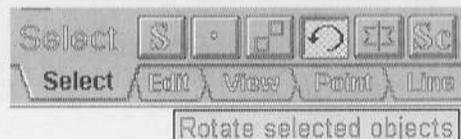
Now we'll need to zoom out to view all of our drawing, the quickest way being the Ctrl + A keyboard shortcut. (A for view All). The inset opening should still be selected. Click now on the "Set the base point" tool, just to the right of the Select tool icon. This will allow us to rotate the selected entities around any point we designate, which in this case will be the absolute center of the entire mat itself.
