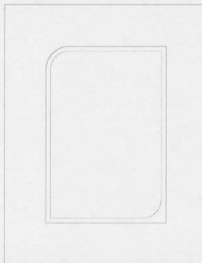
To create a corresponding radius in the top (black) mat layer, click on two of the lines you'll be joining and enter a radius that is  $\frac{1}{4}$ " larger than the first one, or 1.25. Do this for just one of the two corners. (see above-right)
