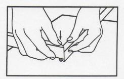
The two sticks of moulding may be adjusted to create a perfect face. We recommend you join three sides of the frame, let it sit a moment to allow glue to set, then complete the frame. Use of a hard, flat work surface is essential. Be sure that all four corners are set—i.e. glue is dry—before continuing.
