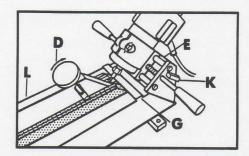
While holding the moulding against both the material stop and the center fence (L), tighten moulding clamp (D) down onto the rabbet of the moulding.
