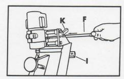
Once the handles have been installed, flip the depth stops (K) down and push the router motor fully from left to right. Make certain that the router bit clears all parts of the equipment.
