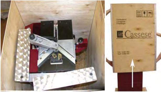
Cut and remove the two ties on the case. Remove the ring from case. Clear the body of case while pulling it upwards. With a flat key of 19 mm, remove the two nuts (E1, E2) under the pallet.
