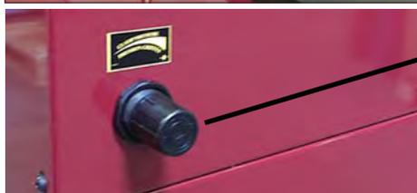
**BUTTON TO ADJUST THE PRESSURE OF THE HORIZONTAL CLAMPS. Minimum allowed pressure is 2 bars. To be used when you replace regular clamps with soft rubber clamps or when you join very softwood moulding.**
