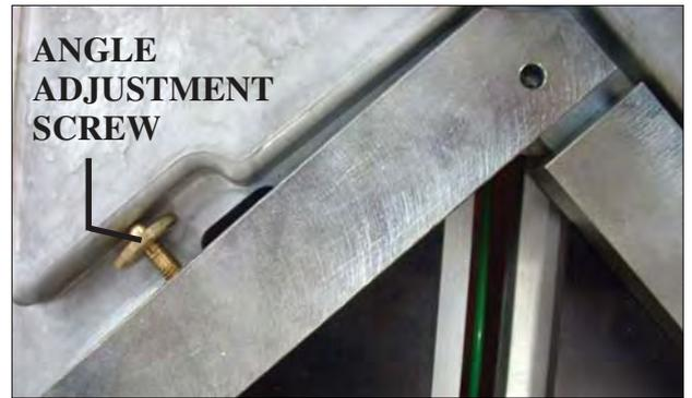
**If the corner is open towards outside, screw in the adjustment screw (see photo page 6 ) for the assembly angle AS (fig 1 p A) to correct the fault and check the quality of the angle by clamping the corner again.**
