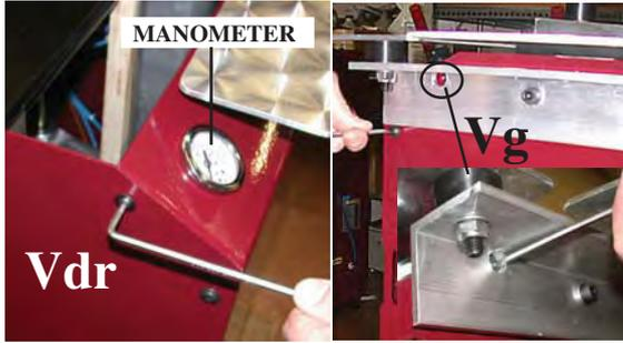
Remove the screws (Vdr, Vg) from the removable front cover of the machine. with a key allen of 4 mm. Make topple the hood. Cut the L ring. While pushing on the arm of pressor, remove the wood piece CB . Loosen the arm of plunger mildly.
