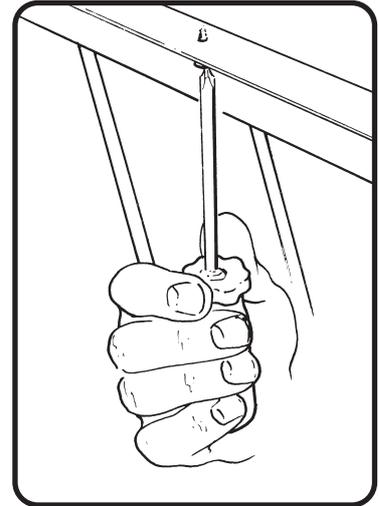
If you are fitting multiple piece worktops, use the **joining plate** (PI01) to fix adjoining worktops as shown. This will prevent a step along the join.
