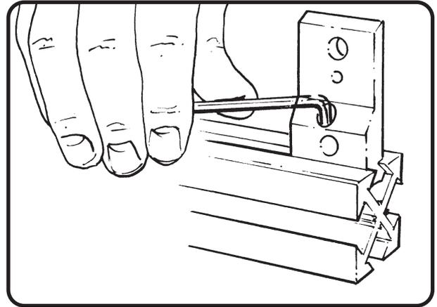
For the reasons described above it is important to locate each component carefully before tightening fully because a small adjustment (*less than 5mm or 3/16"*) will be difficult afterwards. Large realignments will present no problem.
