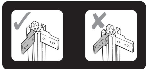
Attach **joining brackets** to the bottom of the **legs**, using a tape measure, or self made spacer to position them accurately to your requirements.
