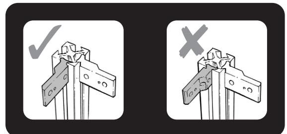
Attach **joining brackets** to the bottom of the **legs**, again using the spacer, position them as shown.
