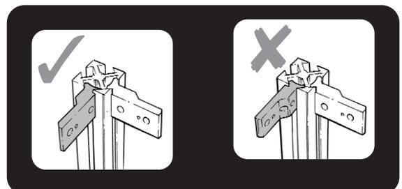
Attach **joining brackets** to the bottom of the **legs**, using the **spacer**. Position them as shown in the diagram. These will make the left & right hand **end frames**
