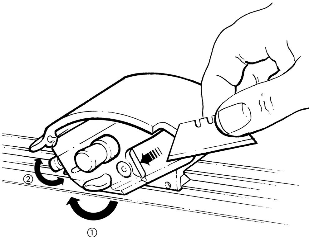
**Inserting and setting the blade**
