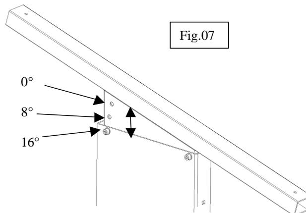
1. Loose the screw (M8 x 16) on the front side of the sidepart.
