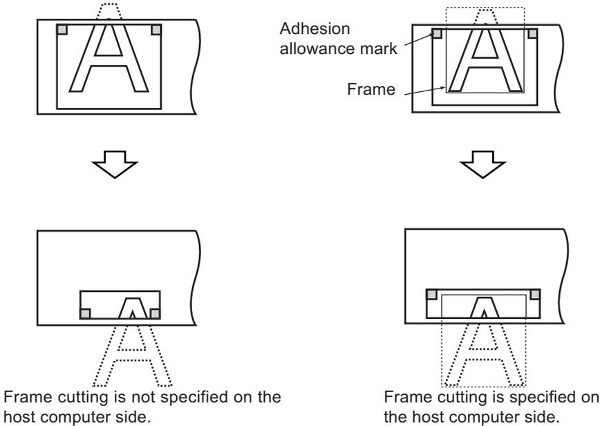
**(NOTE!)** \* The sheet has an adhesion allowance of 1 cm. It is, therefore, necessary that the effective cutting area shall be wider than 1 cm at all times.
