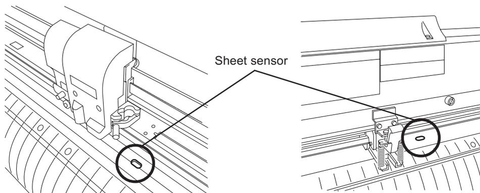
In the case where any of the following types of sheet is used, the sheet sensors will not be able to detect it to give the error message shown below.
