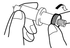
$$\text{Cut in amount} = \frac{(\text{Film thickness} + \text{Base paper thickness})^{*1}}{2}$$
