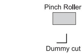
Execute dummy cut this side of the pinch roller that is located near either end of the sheet as observed from the current location of the carriage.
