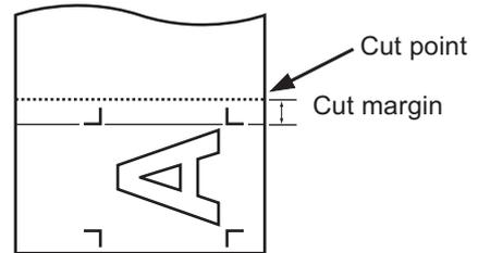
In case detected the distance from the TP2 and the TP1 registration mark during copying the registration mark continuously, cut off the sheet in between TP1 and TP2.
