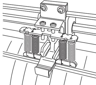
Low mode : Lower the clamp pressure lever.
