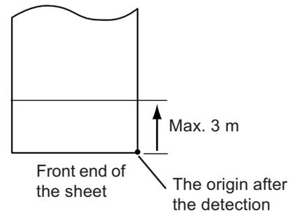
When detecting the rear end of the sheet
