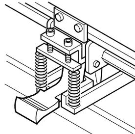
Low mode : Lower the clamp pressure lever.
