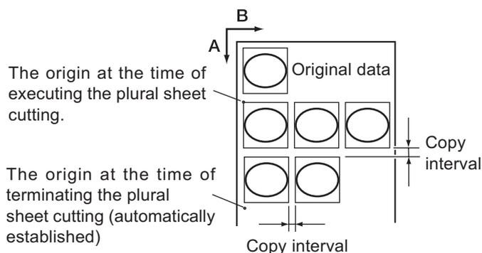
The locations of copies for second cutting (plotting) and beyond are to be allocated according to the size of the original data.
