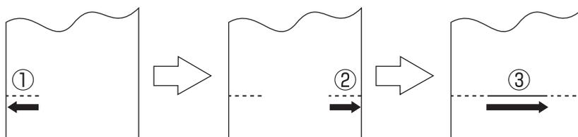
For the two steps cutting, the right part is cut off after cutting 10 cm of the left side.
