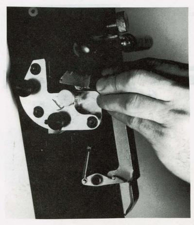
Clamp the glass in place, and raise the cutting head above it. Lower the glass tool by depressing and releasing the blade trigger. Note: The blade holder is not designed to "lock down" in the glass cutting position. Pull the cutting head over the material at a speed of about 1ft. per second. (The glass wheel will automatically begin scoring at the top edge of the glass.) Consistent speed is important for an even score.
