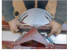
Before every cutting operation bring the protective screen as near as possible to the moulding to cut. Before pressing down and releasing the pedal, never forget to put the two hands on both sides of the shielding caps, on the moulding, <u>far from the knives</u> in order to get a sustained pressure on the moulding while maintaining rabbet ( rebate ) holders.
