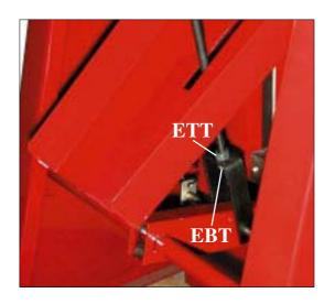
After many sharpening operations, knives might become too short, that means the position of the knife holder related to the pedal has to be adjusted. Press down the pedal and lock it with the aid of the operating handle (MP) ( see page 3).
