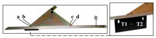
The measuring device is fixed by two threaded holes located on the back side of the table extension.
