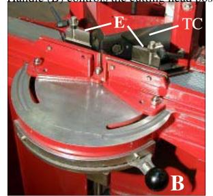
When handle (B) located in the front part of the table is in right end position, the cut is carried out in a single pedal stroke.
