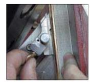
Finally lock screw (B). It is essential to maintain the moulding until rod (A) is locked.
