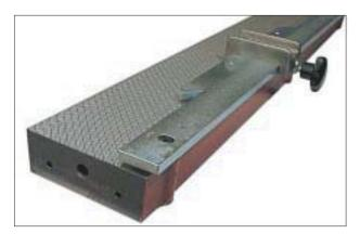
Make sure the both sides coming into contact are cleaned, especially in place of the two pins and of the threaded hole so that the table extension lies level with the table.
