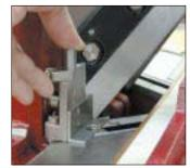
Unlock locking screw (B), push down rod (A) to bring sash angle (C) close to cutting plane....
