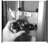
Lift, turn 90\* clockwise, and lower the knife head.
