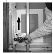
Place the mat face down firmly against the guides in the lower left and close the hold down.
