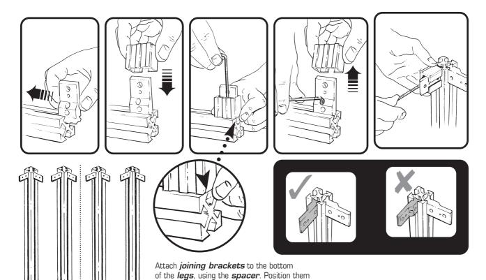
as shown in the diagram. These will make the left & right hand *end frames*
