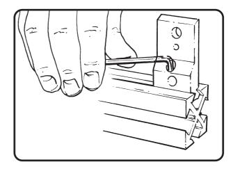
For the reasons described above it is important to locate each component carefully before tightening fully because a small adjustment (less than 5mm or 3/16") will be difficult afterwards. Large realignments will present no problem.
