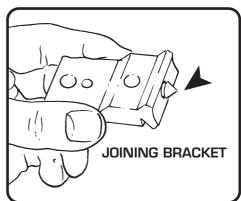
2 Attach the *joining brackets* to the *legs*.
