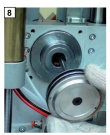
Grease the hammer piston and seals well then insert in the relative hole taking care not to pinch the lip seal. If insertion proves difficult, it is advisable to remove the L-shaped support, the head and V-nail cartridge.
