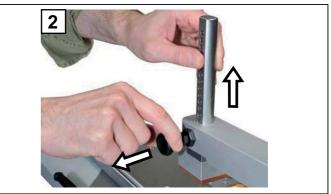
2. If necessary, to overcome the locking knob on the mobile fence, lift the vertical clamp by pulling out the spring-loaded knob.
