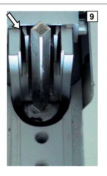
9. NB: align the hammer so that the high part of the piston has the 2 raised sides pointing towards the magazine.
