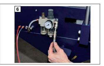
6. Connect up the compressed air supply and adjust the pressure to at least 6 bar, checking the reading on the pressure gauge.
