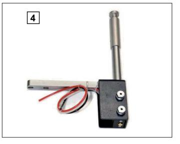
4. The dismantled handle appears as shown in the photo with 3 pipes (black, white, red) connected to the button activated pneumatic valve.
