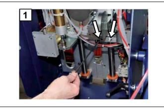
1. Remove the 2 screws which secure the lever to the carriage.
