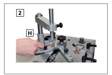
4. Position the magnetic accessories under the pressure plate and check the correct position by inserting mouldings to be joined.
