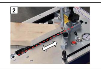
4. The mouldings may have an outer edge which slants slightly. To achieve better contact between these mouldings, the slant along the contact edge of the guides can be adjusted. Turn the knobs as shown in figure alongside to achieve the correct contact tilt in relation to the working bench.
