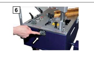
6. Press the cartridge in fully until it locks into position.
