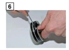
Remove the seals from the hammer, clean well and grease, check for signs of wear and/or splintering. Install new seals taking care to position the lip seal the right way round.
