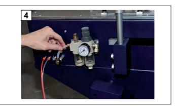
4. Connect the filter to the machine with the compressed air line.
