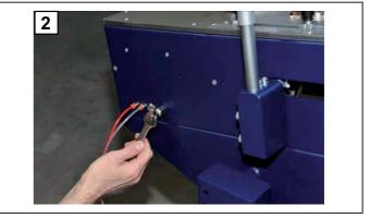
2. Screw in the compressed air line connector.
