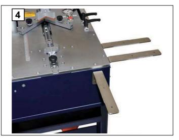
4. After installing all 6 brackets, put the wooden word surface on top and adjust the height of each bracket as required.
