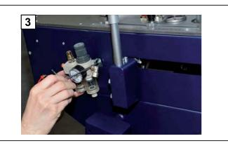
3. Secure the unit in place with the 2 Allen screws.
