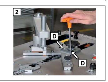
3. Once the screws (D) have been taken out, remove the fence unit.
