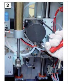
Disconnect the 2 pipes connected to the cylinder Remove the 4 Allen screws which secure the pneumatic cylinder to the head.
