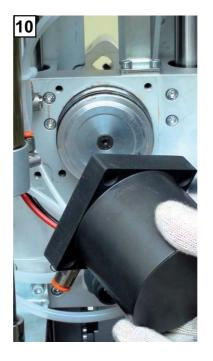
Replace the cylinder and push it well up against the head.
