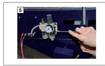
5. Screw the quick-fit connector into filter inlet.
