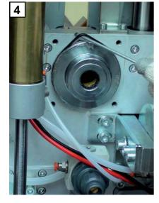
4. Replace the external head seal using a screwdriver to facilitate the operation.
