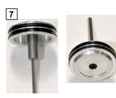
7. It the hammer is worn out or splintered, proceed to replace the whole piston. The raised ends of the hammer must have marked edges to ensure correct insertion of the V-nails.
