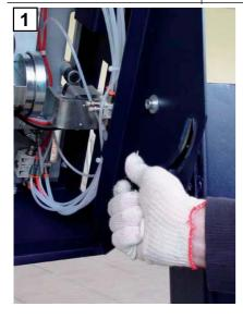
Slacken the locking handle on the support stand to tilt the working bench backwards.
