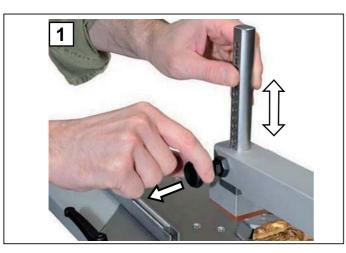
3. Once the new mechanical pressure plate or magnetic pressure plate holder has been installed, tighten the Allen screw.
