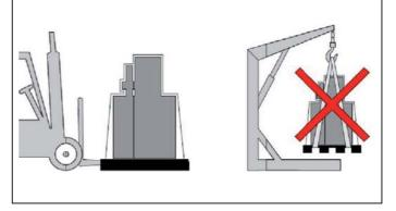
When storing the machine, never stack two machines packed on a pallet with shrink wrap.
