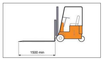
The forks on the equipment used to lift and handle the machine must be in good, undamaged condition and be at least 1500 mm long.
