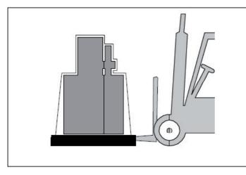
When the machine is packaged on a pallet it must be moved by a forklift.
