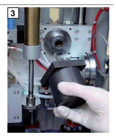
Remove the pneumatic cylinder and extract the hammer which may still be stuck inside.
