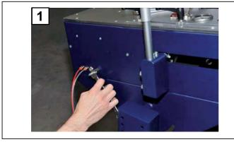
1. Remove the quick-fit connector.
