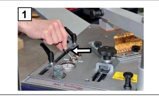
1. Switch the PLV valve (1) lever to the OFF position to open the V-nail pusher.
