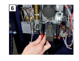
6. Secure the handle to the carriage using the 3 screws and connect the pipes to the exact same connectors as before.
