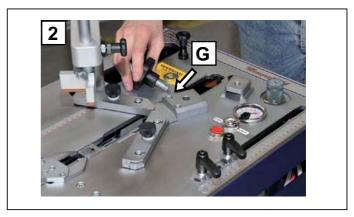
2. To replace the pressure plate, undo the screw (H) which secures it to the rod and pull it off downwards.
