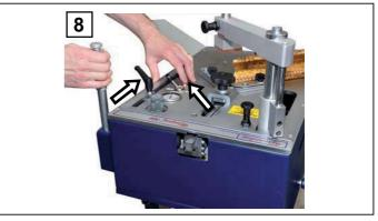
8. Press the red button to move the carriage back within the travel stops and reposition the vertical clamp.
