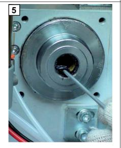
5. Replace the internal lip seal on the head, using a screwdriver to facilitate the operation.
