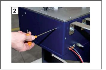
2. Remove the grub screws from the machine casing.
