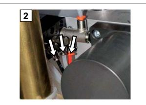
2. Extract the 3 pipes from the connectors, taking care to remember the exact position of each one (black, white and red).
