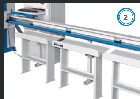
Sorting unit with photocell c/w 3 kickers 3000 x 100 mm
