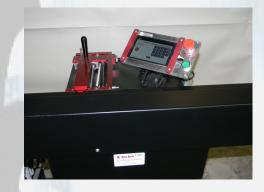
**Manual Measuring Table** 96" with measuring scale and mechanical stop and support stand. *Measuring tables can be produced for most lengths required*
