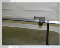
**Vertical or Horizontal Clamping** can be easily added to the machine from the factory or added after the machine purchase. The MN355 is pre-plumbed for this option as a standard feature. *Horizontal clamping may limit the maximum width of cutting capacity*
