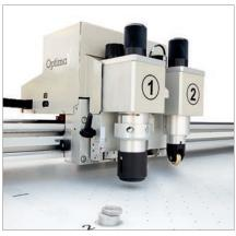
With **two configurable tool stations**, the Optima V is a medium-format professional cutting plotter capable of: Cutting, Half-cutting and Creasing; Drawing and Oscillating Cutting up to 20 mm (3/4") in thickness.
