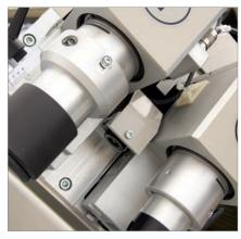
The Optima V comes as standard with a camera for crop mark detection. This device, used in combination with optional software OptiCrop, can perform accurate contour cutting and creasing around preprinted media even with print-distorted materials.
