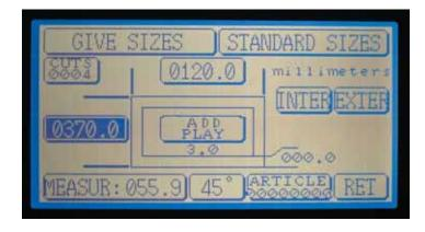
The moulding measurement will be displayed in the MEASUREMENT key (032.1 for example). The measurement is validated by touching the MEASUREMENT key and it will be used to compute the required position.
