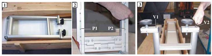
Open the crate and put the NS foot stand into an upright position. With a 4mm hex head key, unscrew the 4 screws of the 2 foot stand locking plates: P1 and P2 . Push P1 and P2 right back with a mallet, then slide them down to the bottom of each foot. Retighten the 4 screws of plates P1 and P2. With a 5mm hex head key, unscrew V1 and V2 and put the NS feet in the outside position as shown in figures 3 and 4.
