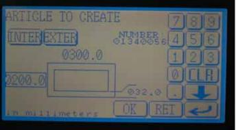
Touch the validation key . The message 'PLEASE WAIT' appears for about 1/2 second then the file data screen appears. You can modify any of the values using the numeric keypad. All the values entered must be validated immediately by touching the key. Use the key to move from one value to another.
