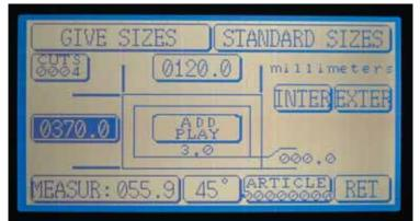
The file parameters displayed in this screen are the last parameters created, modified, listed or executed. This means that after a machine power failure, you do not need to re-enter a reference before resuming work. Also, you can list the file that you are interested in and then execute it without having to call up its reference.
