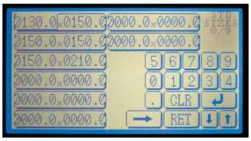
A frame is executed by touching its key: the execution screen will appear, allowing only the length and width values of the standard frame to be adjusted.
