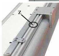
Unlock locking screw Z and slide the guide GB of the NS along screws 1-2-3 of the right-hand table and the nuts of the 2 ruler supports R1 and R2. Screw 3 should be visible in hole T3. Tighten screws 1, 2, 3 and V1 and V2 of ruler supports R1 and R2 with a 4mm hex head key.
