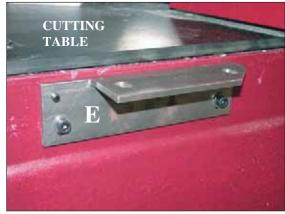
Take the NS out of the crate and turn it over. Place the bed of the NS on bracket E, and screw them together (10mm long tubular socket wrench + 5mm hex head key) **without tightening**, with the 2 screws, 2 washers and 2 nuts provided.
