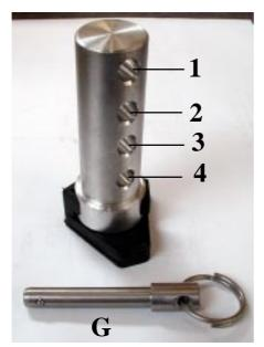
This new version top presser comes now with your CS 79 as a standard feature. Its height can be adjusted with the pin so that the machine can work up to 78 mm (3"1/8) tall mouldings. Pay attention to keep always maximum 30mm (1"1/4) distance between the top presser and the mouldings and to keep the rubber triangle parallel to the 90° angle assembly (backfences B1 & B2, Fig.1, p. 1)
