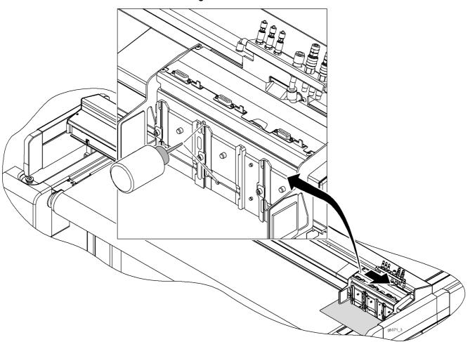
Fig. 7-11 Lubricate bearing
