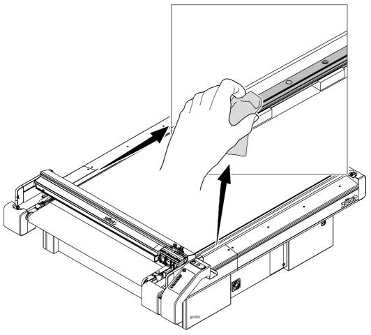
Fig. 7-5 Oiling the guide rails
