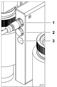
Fig. 4-21 Connection - electrical tools
