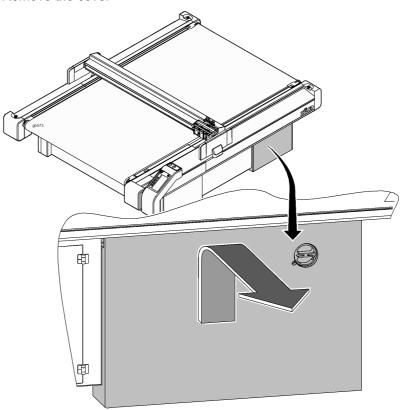
Fig. 7-15 Remove the cover
