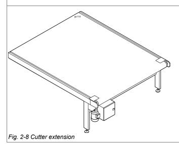
Cutter extensions guarantee efficient working. The material supply/removal is carried out while the cutter is completing its jobs. These extensions are available in different sizes, either with or without auxiliary drive.
