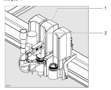
Fig. 5-10 Tool slot, tool assignment e.g. Module 2, tool 1
