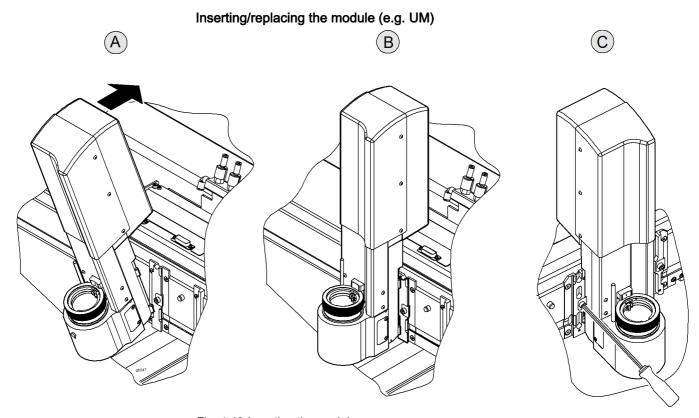
Fig. 4-19 Inserting the module
