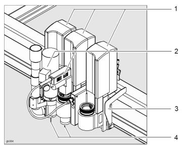
Fig. 4-17 Module carriage/module/tool/knife, router etc.
