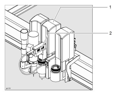
Fig. 5-12 Tool slot, tool assignment e.g. Module 2, tool 1
