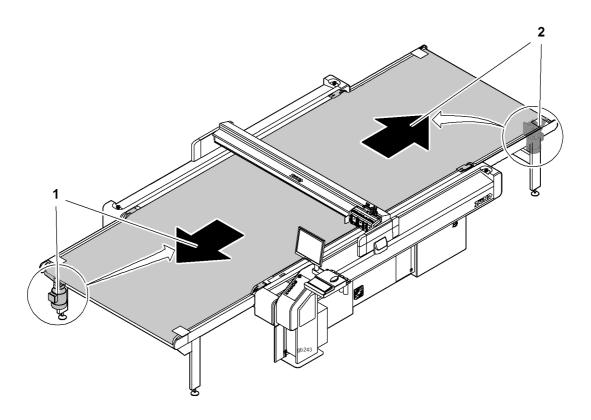
Fig. 4-27 Feed direction - position of auxiliary drive
