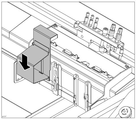
Fig. 4-36 Slot protective plate
