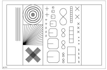
Fig. 5-22 DIN test, 255 mm x 170 mm
