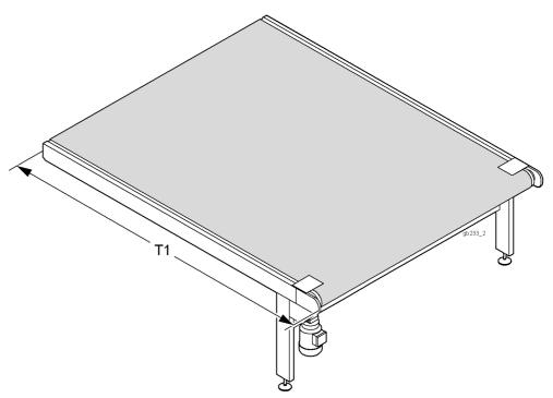
Fig. 2-10 Cutter extension dimensions
