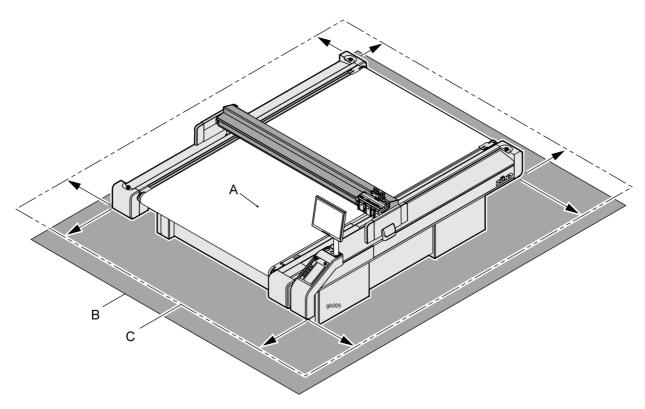
Fig. 3-4 Working area around the cutter
