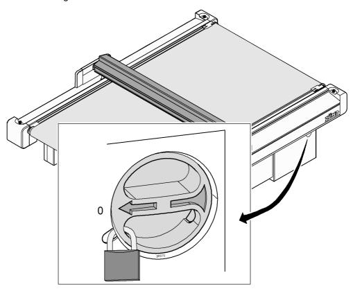
Fig. 7-3 Secure the machine
