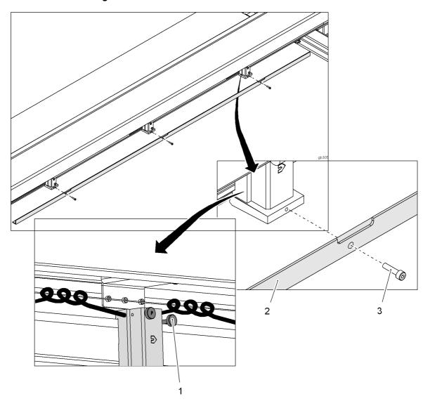
Fig. 4-29 Feed guide rail
