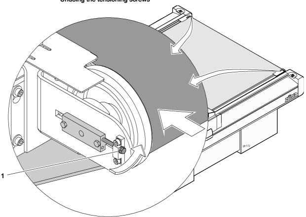
Fig. 7-17 Undoing the tensioning screws
