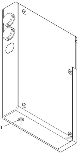
Fig. 4-33 Laser pointer settings
