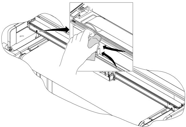
Fig. 7-10 Cleaning the guide rails
