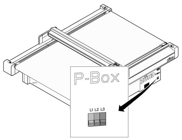
Fig. 7-16 Automatic circuit breakers
