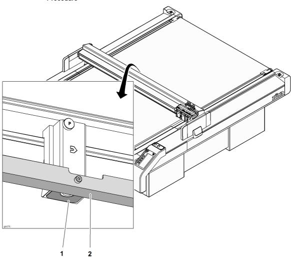
Fig. 7-13 Cleaning the feeding clamps/feed guide rail
