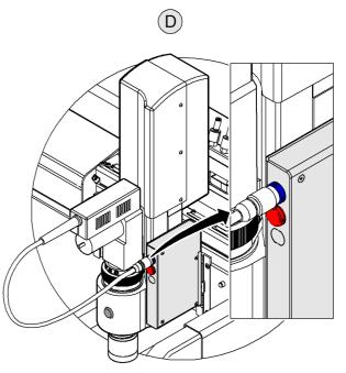
Fig. 4-20 Inserting tool
