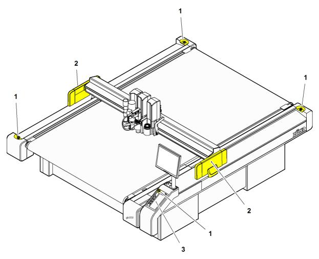
Fig. 3-6 Safety and monitoring devices
