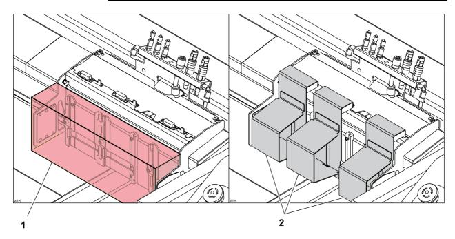
Fig. 3-2 Danger area on the module carriage
