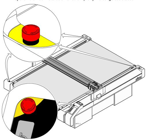
Fig. 4-8 Emergency stop switch
