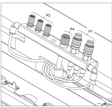
Fig. 4-22 Interface unit - connections
