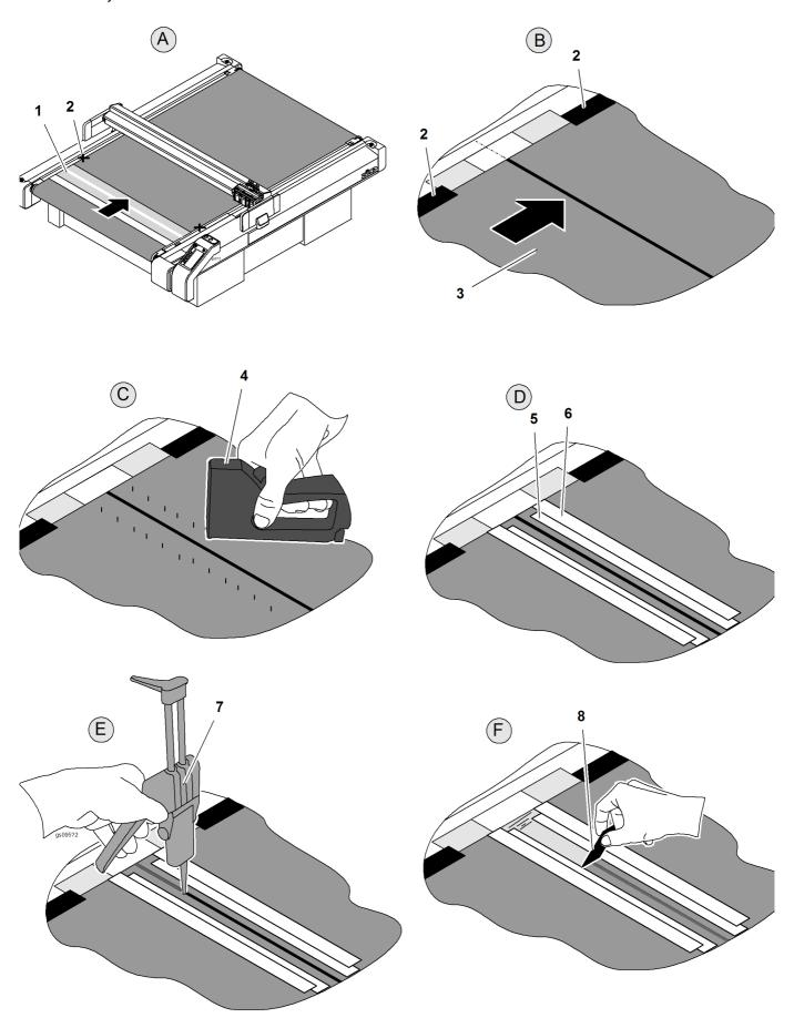
Fig. 7-22 Gluing the conveyor belt
