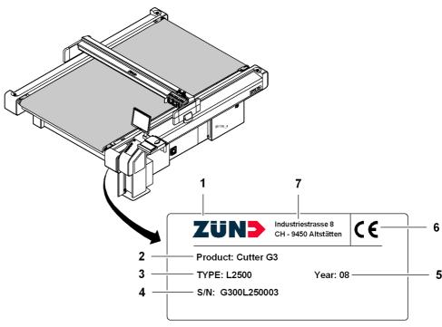
Fig. 2-2 Position of rating plate
