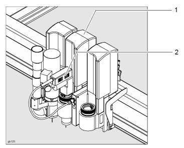
Fig. 5-7 Tool slot, tool assignment e.g. Module 2, tool 1
