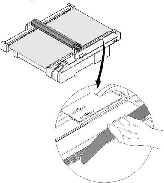
Fig. 7-12 Clean the chipping protection brush
