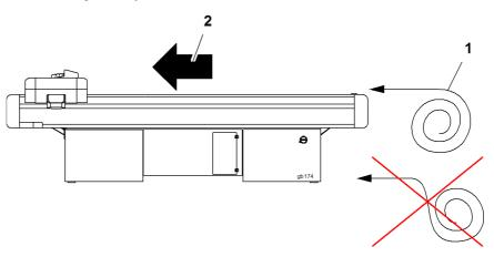
Fig. 7-19 Determining conveyor direction
