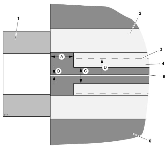
Fig. 7-21 Overview - gluing the conveyor belt
