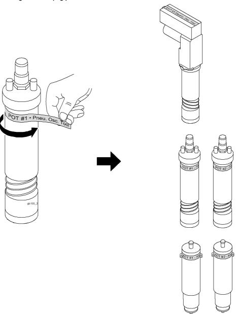
Fig. 4-16 Marking the tool (e.g.)
