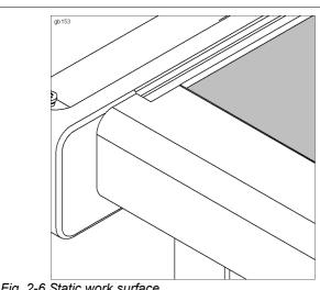
The feeding and removal of the processing material takes place on the work surface of the cutter. The work surface is protected against damage using a cutting base.
