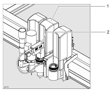
Fig. 5-14 Tool slot, tool assignment e.g. Module 2, tool 1
