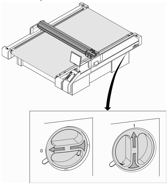
Fig. 4-12 Switching on the machine
