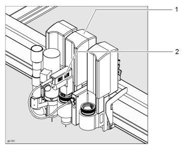
Fig. 5-8 Tool slot, tool assignment e.g. Module 2, tool 1
