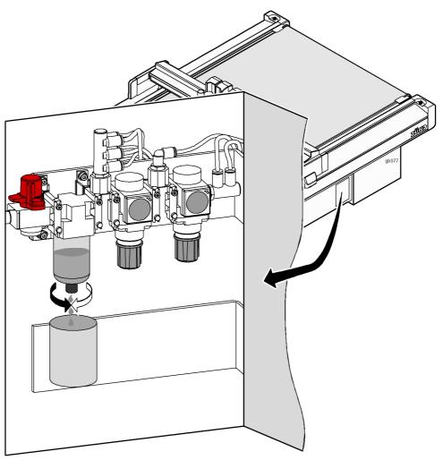
Fig. 7-14 Drain condensation water
