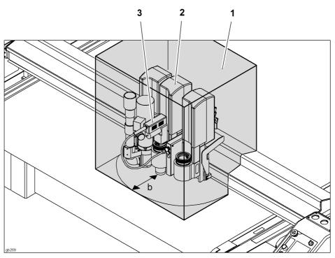
Fig. 3-3 Danger area during the installation
