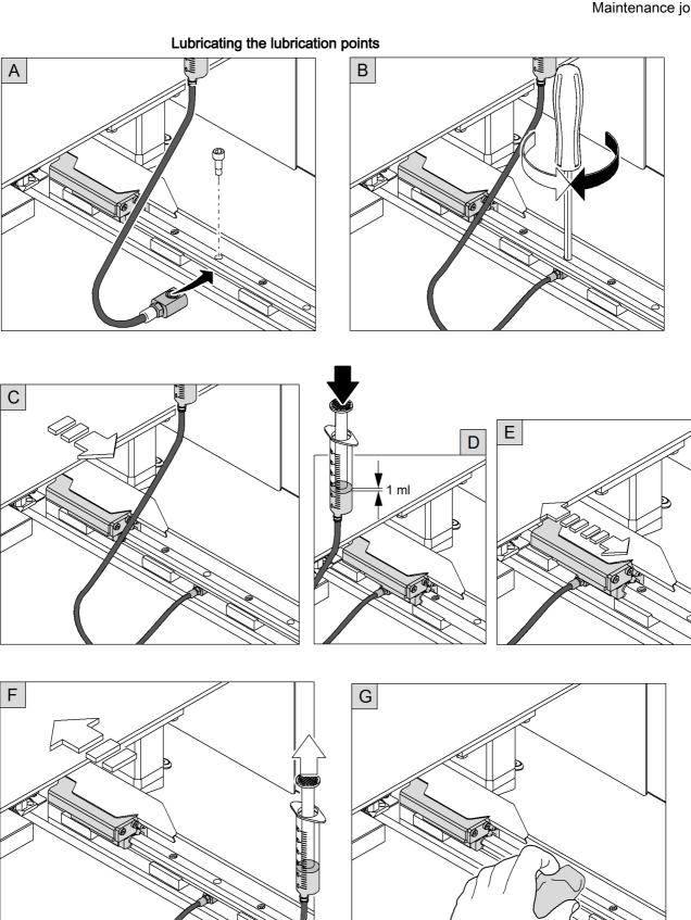
Fig. 7-8 Lubricating the lubrication points
