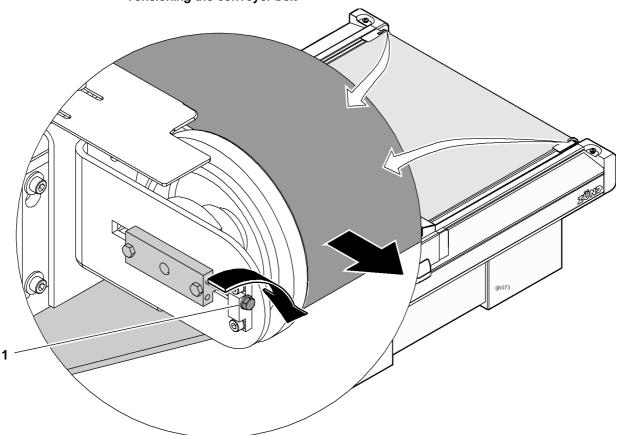
Fig. 7-24 Tensioning the conveyor belt
