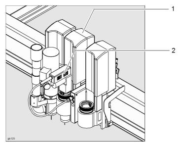
Fig. 5-2 Tool slot, tool assignment e.g. Module 2, tool 1
