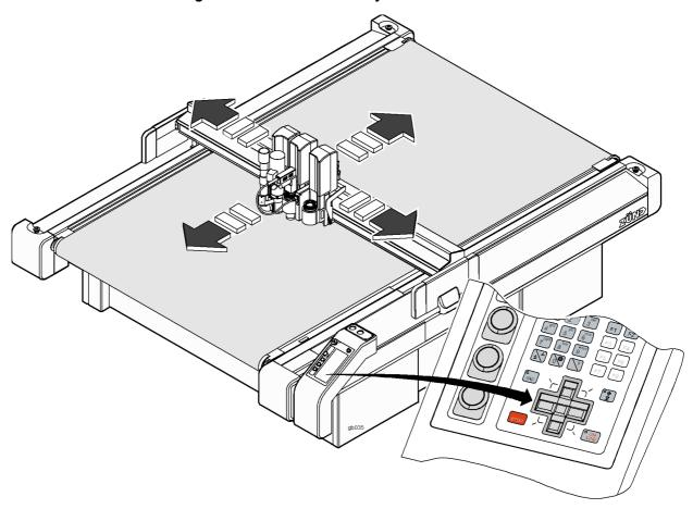
Fig. 4-14 Moving the bar/module
