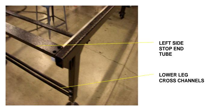
With both the Left and Right rail sections attached and level, position the loading table that was shipped separately from the press. This is done by rolling the loading table into the rail section from the proper end. This is determined by the loading table that was already on the press when shipped.
