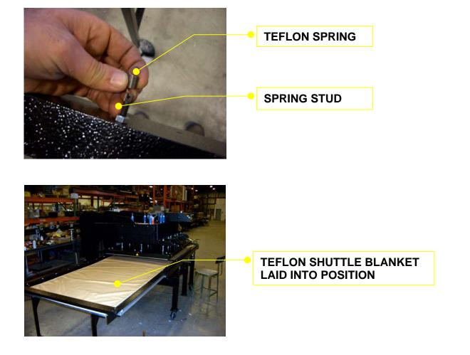
With the Teflon blanket now secured, shuttle the assembly to the left and right. Make sure that the Teflon slides smoothly without risk of abrasion against edges or surfaces. In most cases the bottom heater block will have a layer of 1/8" green heat conductive rubber laying on top of the heater block surface. The Teflon blanket needs to be above this green heat conductive rubber/semi porous Teflon by approximately ¼".
