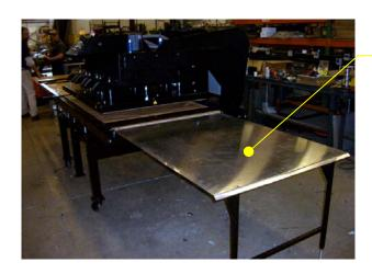
ALUMINUM SHEETS ATTACHED TO THE OUT-RIGGERS ONCE ATTACHED. SCREWS FASTEN THE ALUMINUM SHEET TO EACH OUT-RIGGER VIA ALUMINUM ANGLES WELDED TO THE TIN AND SCREWS THAT SCREW INTO THE 1" X 1" STEEL
