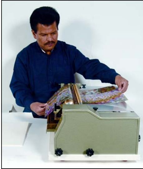
COLONEL applies adhesive to back of label. Operator places label onto board stock.
