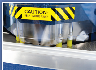
T-400 contains four pneumatic hold down clamps for securing moulding
