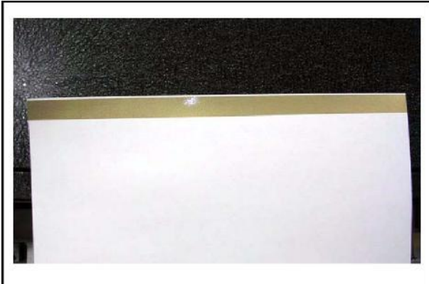
Fig. 3-55. Adjust Until Tracking is Even Across Top of Paper Edge
