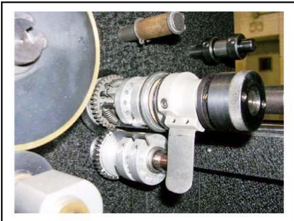
Fig. 4-24. Rotate Housing So Blades Start to Separate
