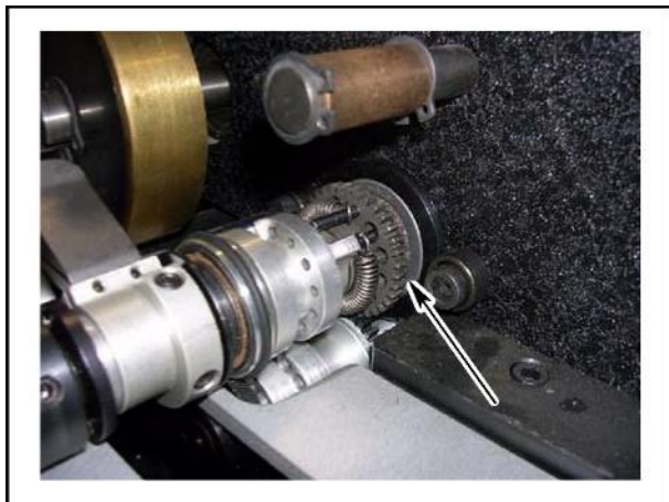
Fig. 4-1. Oil Cutting Package Gears
