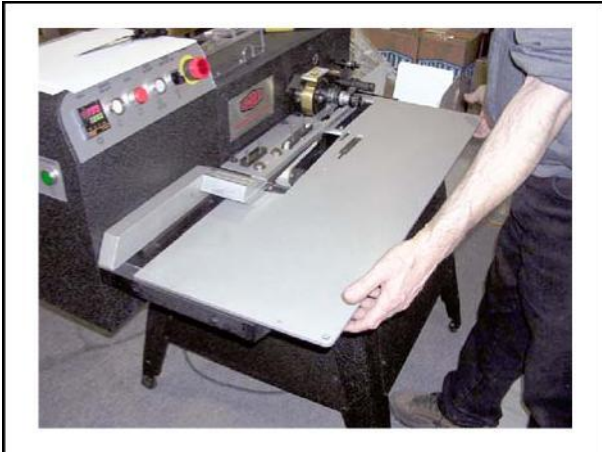
Fig. 3-34. Lift Table Off Locating Pins
