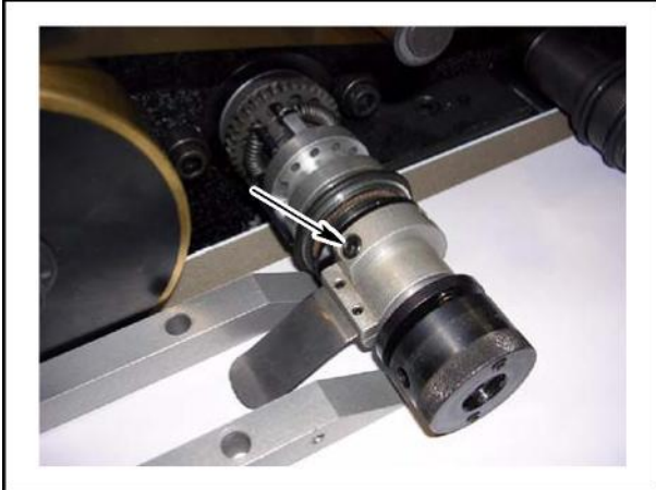
Fig. 3-25. Loosen Guide Finger Set Screw
