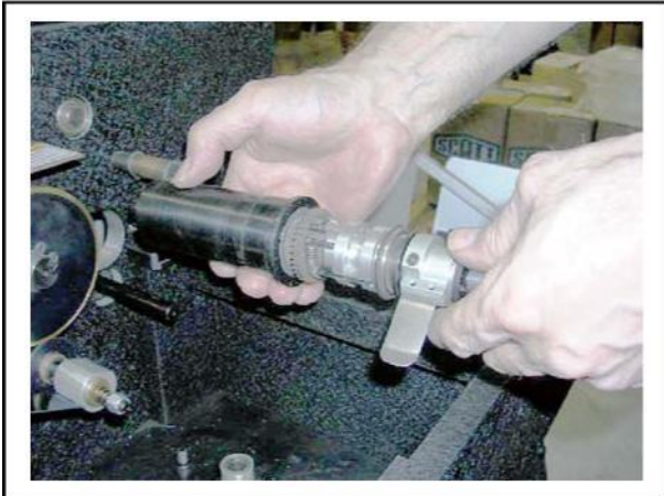
Fig. 4-20. Rotate the Housing So That Blade Can Move Freely Between 6-9:00 Position
