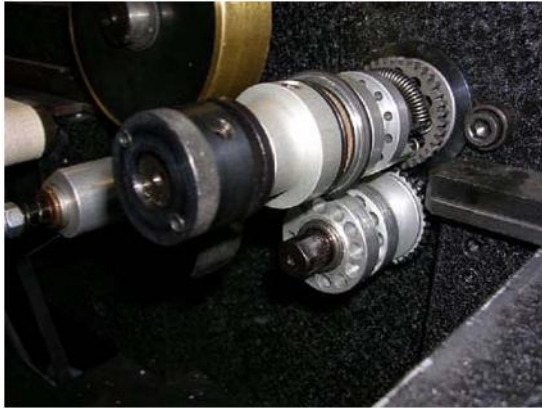
Fig. 4-26. Rotate the Lower Cutter into 2:00 Position
