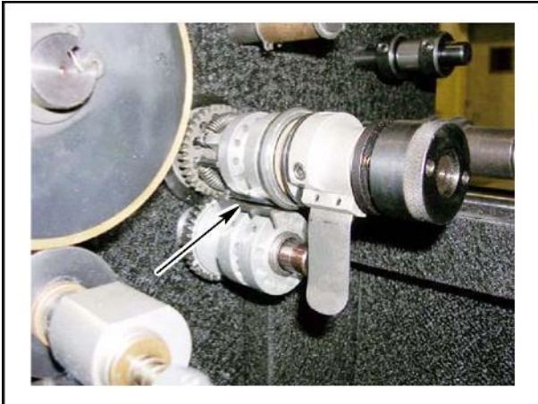
Fig. 4-23. Install Lower Cut Off - Blades Ready to Cut
