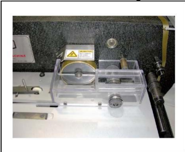
Fig. 1-10. Burn Hazard - Heat Rollers
