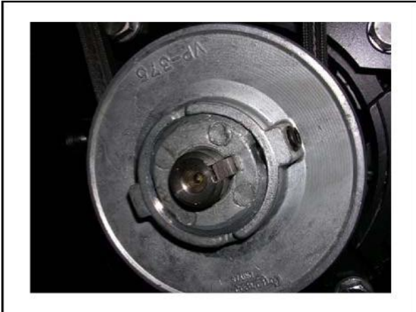
Fig. 3-40. Rotate Pulley Hub 1/2 to 1-1/2 Turns
