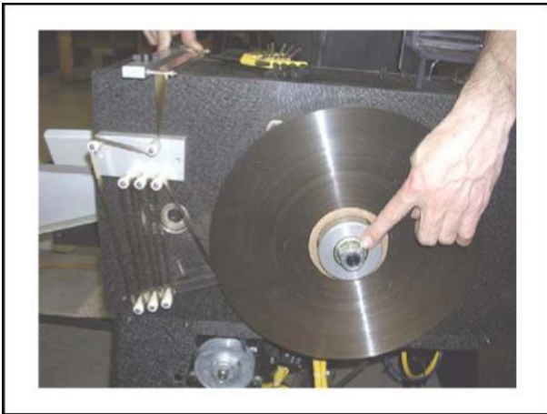
Fig. 3-36. Adjusting Auto Brake on Reel Holder
