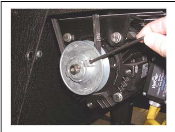
Fig. 3-39. Loosen Set Screw in Pulley Hub
