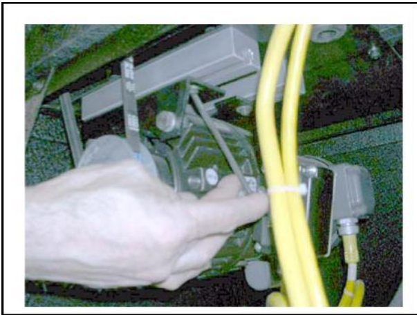
Fig. 3-38. Loosen Drive Motor Mounting Bolts
