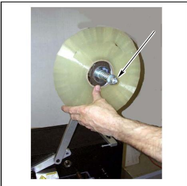
Fig. 3-48. Install Self Adhesive Tape as Shown
