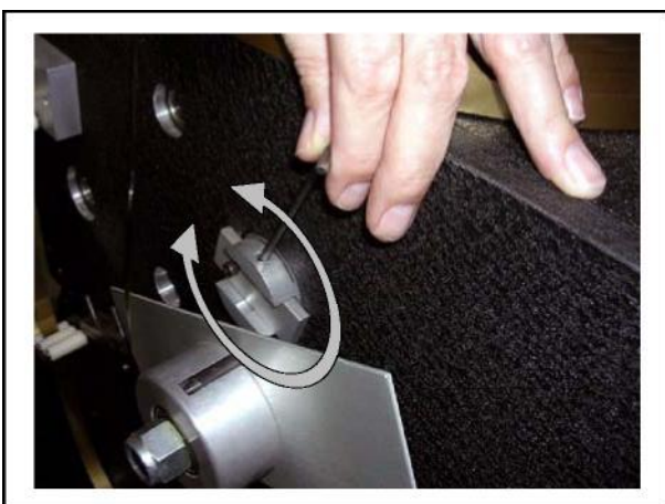
Fig. 3-54. Rotate the Holder Slightly to Adjust the Pitch of the Heat Roller
