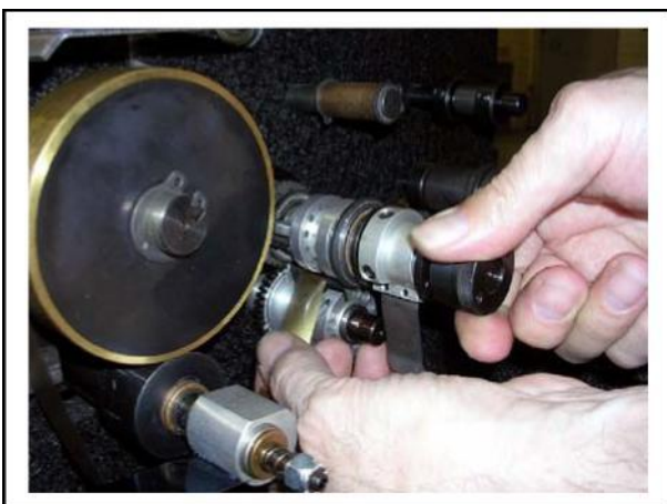
Fig. 4-25. Test Blade Positions By Cutting Tape
