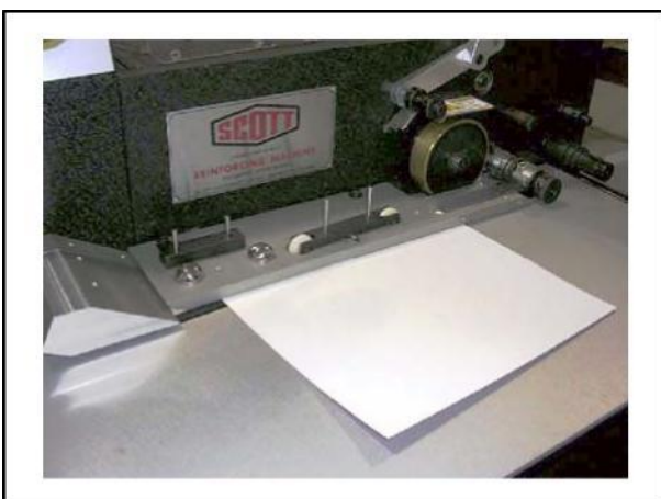
Fig. 4-11. Insert a Sheet of Stock to Depress Trip Switch
