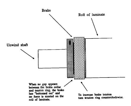
NOTE: When reloading rolls of laminate, reset the brake to 0 (hottomed out).
