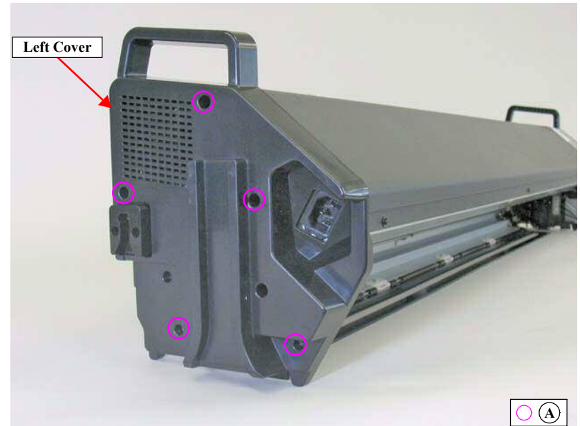
Figure 4-198. Removing the Left Cover
