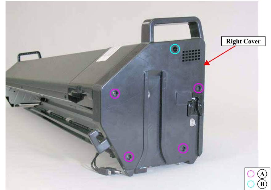
Figure 4-197. Removing the Right Cover
