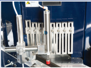
Pneumatic Hold Down Part Clamping Mechanism
