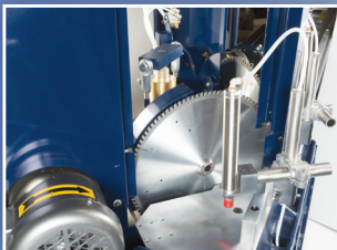
Inside Cabinet View of Saw Blades and Motor Assemblies
