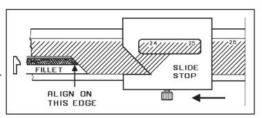
**STEP 2 b:** If you're measuring by hand, place the cut fillet under the mat so that the cut end will fit into one corner of the opening. Hold the fillet in place with one hand and use the other hand to mark the fillet with an exacto knife or a used mat cutter blade. Make the mark straight across the fillet. Remove the fillet from under the mat and continue the mark using the blade to make it easy to see.
