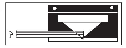
**STEP 2 a:** If you're using the measuring arm, after making your first edge cut, slide the fillet over to the 45° *ANGLED* line that matches the dimension you want to cut. (Use the vertical step in the fillet to measure.) Bring the Slide Stop over to touch the fillet edge. Fingertighten the screw on the stop. Check the cut piece of fillet in the mat opening for trimming to **exact** size.
