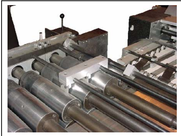
Fig. 3-18. Correctly Set Space Between Upper & Lower Rollers
