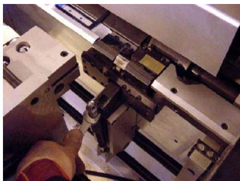
Fig. 4-75. Use an Open Ended Wrench to Compress Spring Pressure on Linkage
