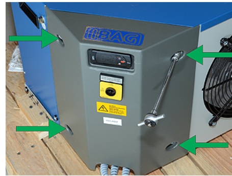
Remove cover (4 screws)
