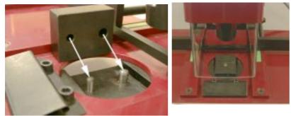
One special bottom stamp for each type of hanger is needed. Install it as shown above on the machine; 2 holes of different sizes corresponding to 2 pins on machine, make sure that you cannot install it badly. 3
