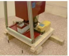
Put the MF20 with its wooden base on higher wood pieces to create a bigger space to remove the screws from underneath; you need a 19 mm wrench.
