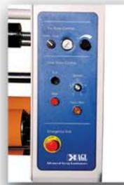
**Logic Control Panels** - The AGL 64i is truly a bi-directional laminator, with full access to the controls you need from both the front and rear. Including speed! We've also included a very useful quick reference guide for material thickness and conversion formulas. Our easy to read and reach controls provide you with constant feed back.
