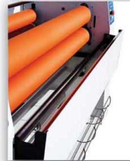
under the table or get on your knees (a laborious task on other laminators). The Easy Web Feed Table also features a dual latch for secure docking, yet has an elegant single handle release making it a smooth and fast one handed operation. Another not so obvious, but strong, feature on the Easy Web Feed Table is the hidden film guide. When the table is in the "dis-engaged position" it exposes the film guide ensuring that
