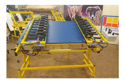
MODEL: STRETCH MASTER PLUS MULTIGUN Stretching Size: 1m x 1m Part No: SMPM40
