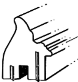
Junction with more parallel and superimposed staples
