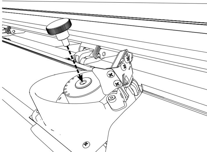
**Figure 16.** Tighten the *Sorter Wheel* thumbscrew.
