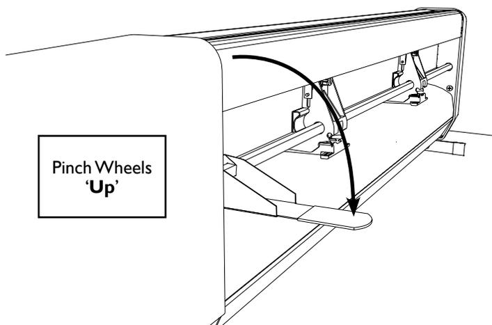
**Figure 25.** The *Pinch Wheel Lever* when wheels are locked up.
