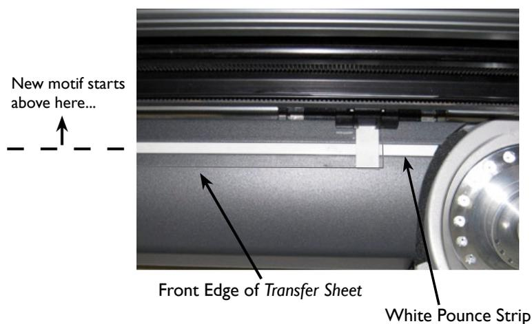
**Figure 27.** Insert a *Transfer Sheet* then lock the *Pinch Wheels* down.
