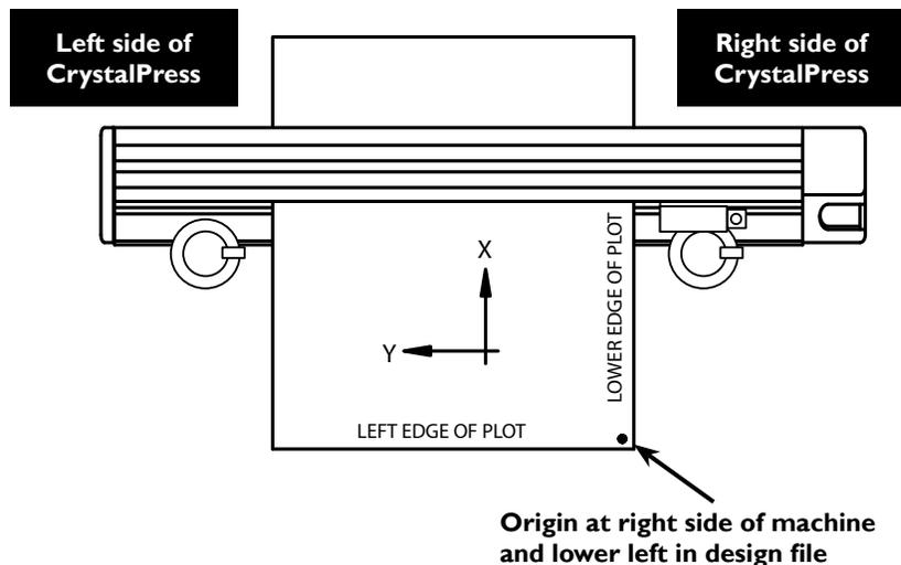
Figure 3. The X and Y axes and origin (top view).
