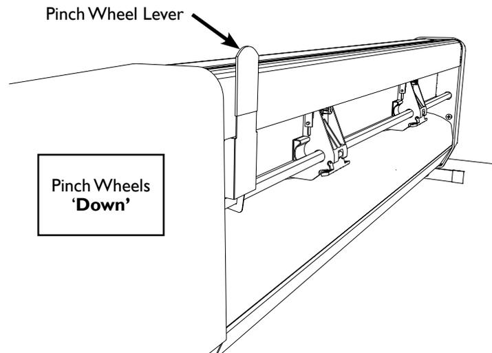
**Figure 24.** The *Pinch Wheel Lever* when wheels are locked down.
