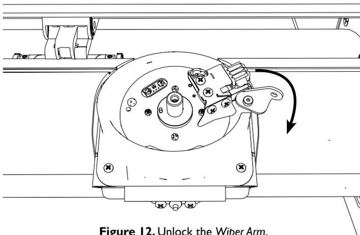
Figure 12. Unlock the Wiper Arm.
