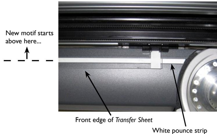
Figure 9. Position *Transfer Sheet* with **Arrow** keys.
