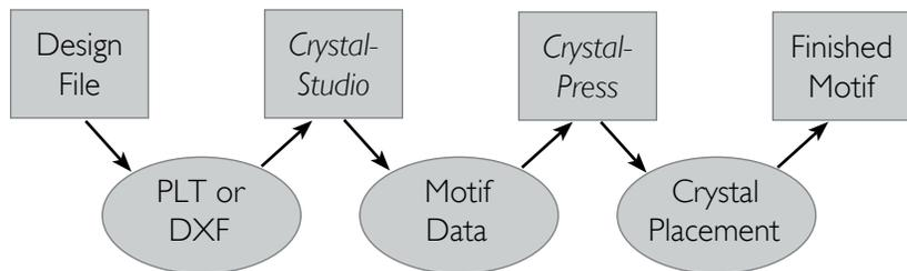
Figure 2. Work flow and data types for making a motif.
