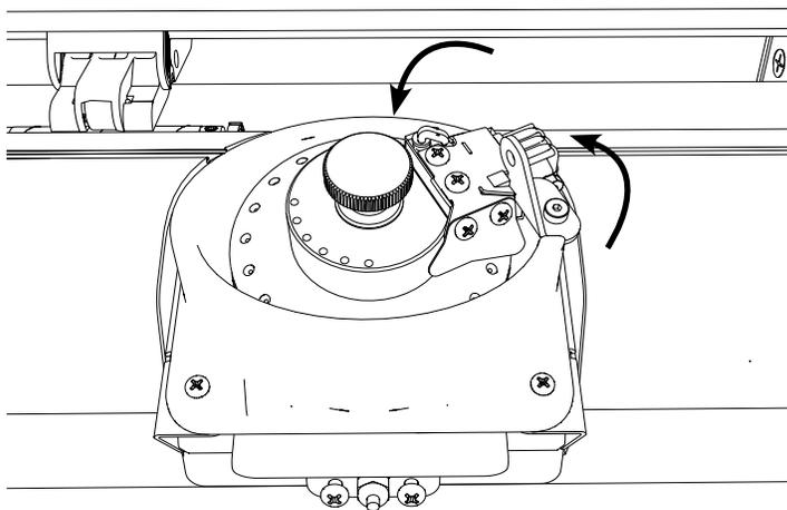
**Figure 17.** Rotate the *Wiper Arm* into place then lock it down.
