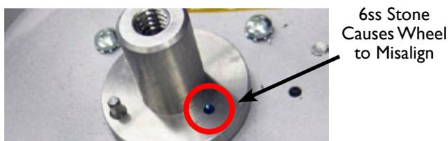
**Figure 39.** Stone trapped on *Sorter Bowl* shaft.
