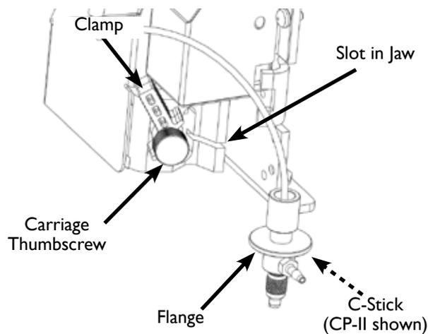
**Figure 19.** Insert the *C-Stick* in the *Carriage*.
