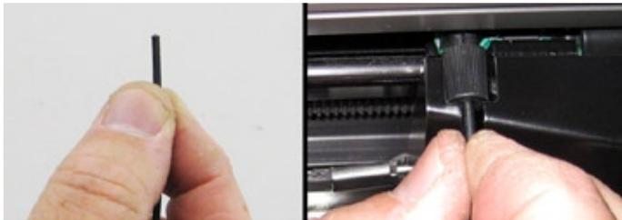
Figure 22. Insert the *C-Stick* cable into the socket.
