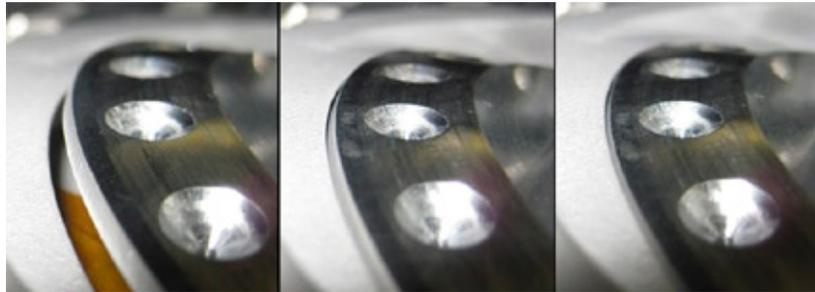
*Sorter Wheel* **not** seated on shaft or large stone(s) under wheel.
