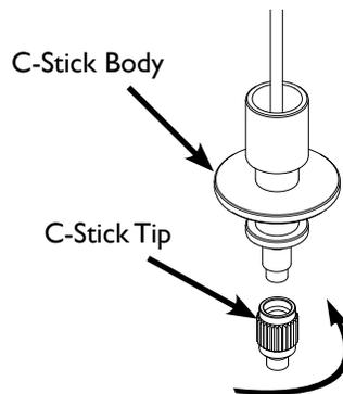
**Figure 18.** Install the *C-Stick Tip* onto the *C-Stick Body*.
