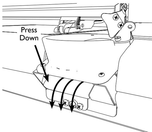
**Figure 30.** Direction of falling stones when *Stone Release Door* open.
