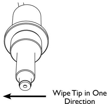
**Figure 37.** The *C-Stick* with tip shown for cleaning.
