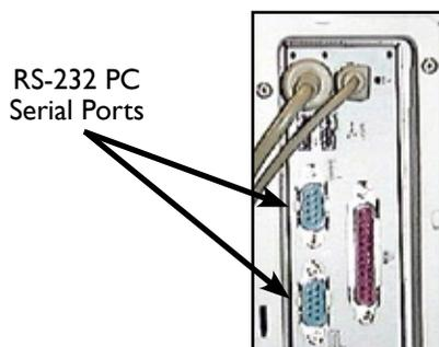
**Figure 34.** Serial Ports on a computer.
