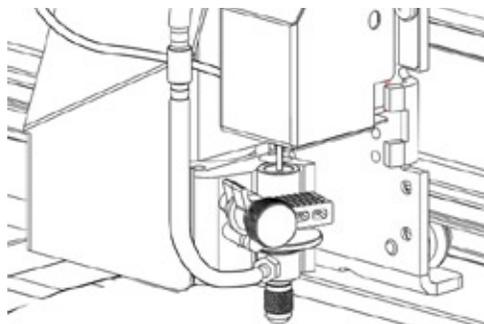
Figure 23. Attach pump hose to tool (*CP-II* only).
