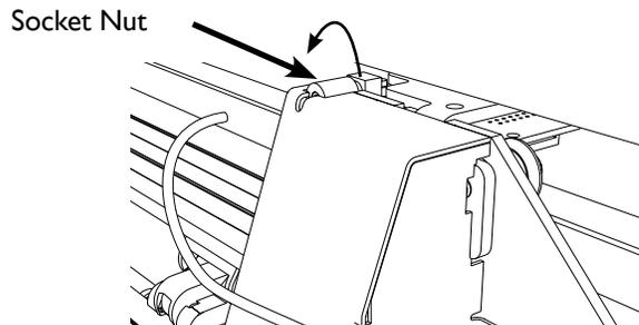
Figure 21. Loosen the *Socket Nut* (*CP-II* pump removed for clarity).
