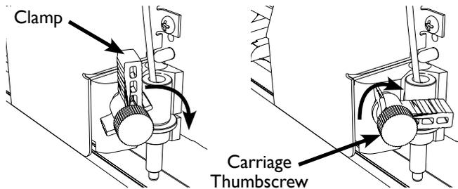
Figure 20. Tighten the *Carriage* clamp thumbscrew.
