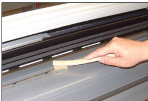
**Figure 35.** Cleaning the *Drive Shaft*.
