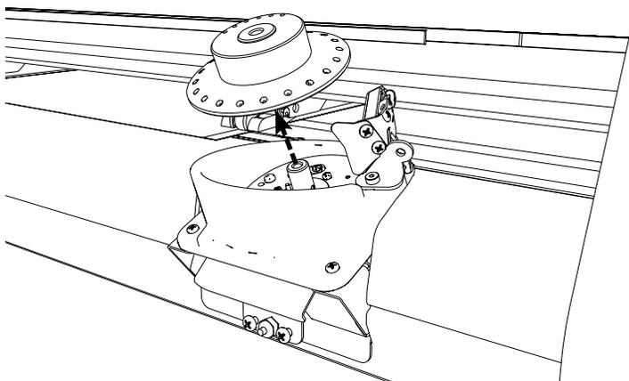
**Figure 29.** Removing the *Sorter Wheel* from the *Sorter Bowl*.
