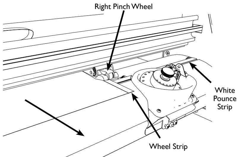
**Figure 26.** Insert a *Transfer Sheet* then lock the *Pinch Wheels* down.
