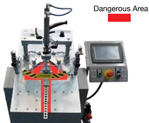
Figure 3.4.A - Working area and dangerous zones
