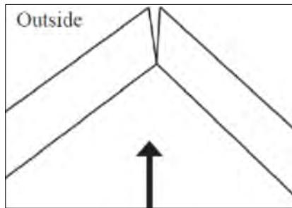
Tighten the adjusting screw to correct the defect of the mouldings.
