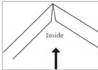
Loosen the adjusting screw to correct the defect of the mouldings.
