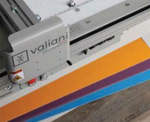
The button clamp system allows to trim the material right to the edges, optimizing the material yield and leaves no more marks on your material. A manual blade depth adjustment dial with increments of just 0.1 mm (1/32") provides much better quality control when working with various materials and thickness. A materials storage is located behind the front plate.
